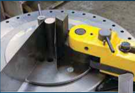
Built Up Forming Nose For forming wider materials with higher collars.
