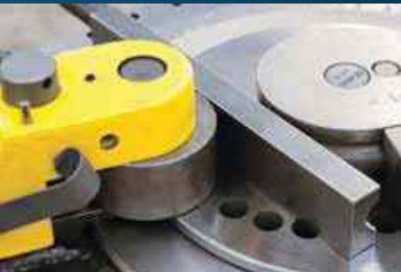
Forming Roller Replaces Forming Nose to eliminate part marking or back up for Follow Block to reduce drag.
