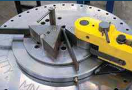
Radius Block - Used with standard Locking Pin; for forming solid material to a tight radius.
