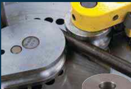
Grooved Forming Roller - Used with Quick-Lok Clamp for forming larger radius in tubular stock.
