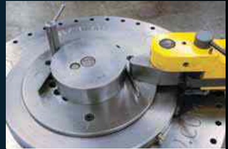
Radius Collar Style B - Used with standard Locking Pin; for forming solid material.
