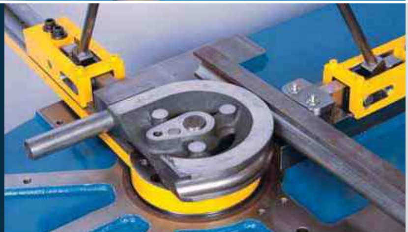
Standard Grooved Collar for bending round tubing. Used with Clamp Block and Follow Block.
