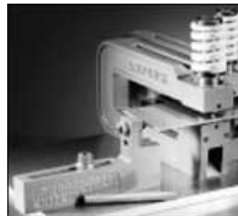
Typical 3-pin gaging Template Mounting
